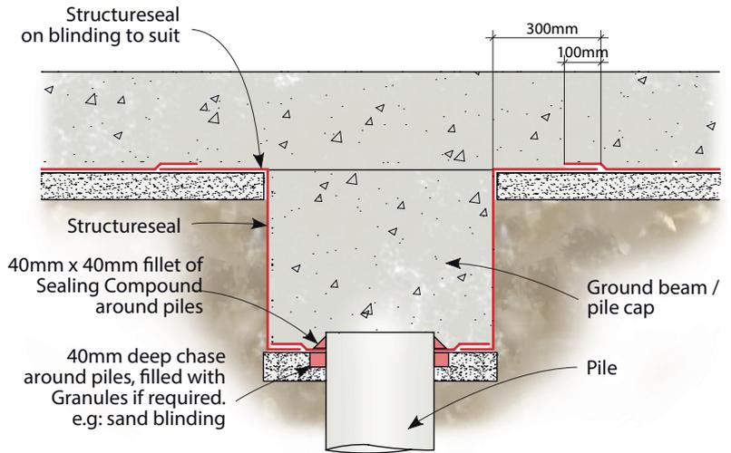
**Detail 2 - Typical Slab Detail at Foundations**
